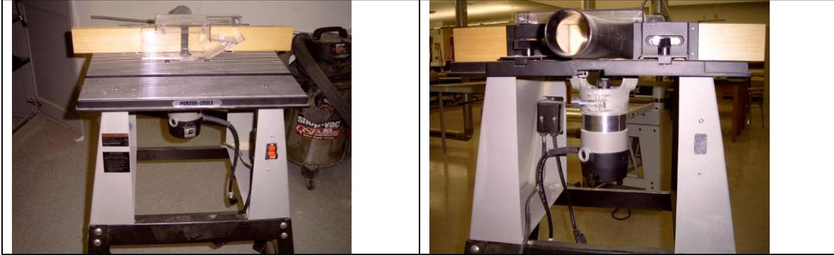
Uses: To create decorative edges or to cut grooves/channels into a piece of wood.
