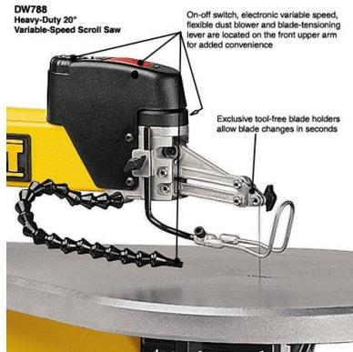
Uses: To cut sharp curves, details, or the inside of a piece of flat material (wood, plastic, etc.).
