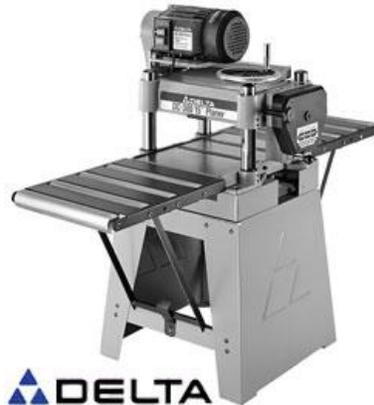
Uses: For shaving material off the plane of a piece of lumber. The planer allows you to machine your piece of lumber to the proper thickness.
