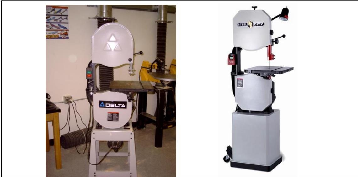
Uses: Used for cutting details, mostly straight lines or large curves in wood or plastic.
